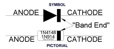
To help you fully understand and identify the markings on the diode(s) used in the ISO-KITS, I've drawn a symbol and picture help the user relate the symbol definition to a pictorial of a diode.
