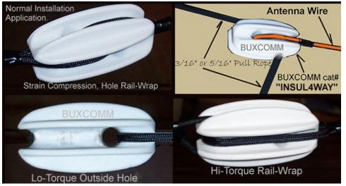
When attaching the BUXCOMM INSUL4WAY insulators, use the method that you feel will suffice with the ends, or corners. Notice that either *end tie-tail wires*, or *UV resistant rope* (BUXCOMM BUX316) can be used to attach the insulator(s) to a pole, mast or tree. Rope can easily glide through the satin finish of the insulators we provide with the 1TRA kit.
