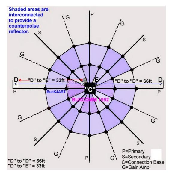
At each end I leave enough wire to connect, or solder, to the antenna ground/base-plate and at the opposite end, I connect to a short copper-clad ground rod (BUXCOMM item# GROUNDROD ) cut into 3 short pieces. I use item# G10701 or G4401.
