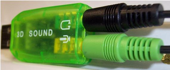
USB SoundCard shown in the example is BUXCOMM cat# (MISO) **NOTICE** the **BLACK** plug is inserted into the **Speaker** jack (with head phone symbol). The **GREEN** plug is inserted into the **MIC** jack (with the microphone symbol). If your sound card does not have a LINE IN jack, use the MIC IN jack to your soundcard. DO NOT use the "Mic Boost" option. Be sure it is NOT enabled (DISABLE IT). This is found by selecting Options on the Player Control > Properties > select Recording OK >
