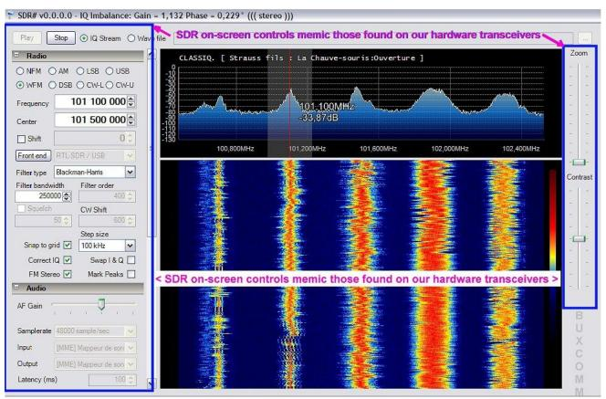
In addition to the display exhibiting the SDR controls and buttons, it also displays a panoramic view of the band on each side of the selected frequency. This panoramic view is several megahertz wide, providing indication of other signals each side of the frequency we are listening to.
