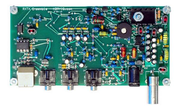
The RxTx SDR transceiver (shown above) comes in five models... The TxRx SDR transceiver kits are in five packaged for various segments of the HF Bands, The list of band segments are:
