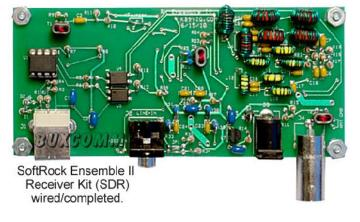
The SoftRock RX Ensemble II Receiver *Kit* (at left) include the components to build the kit for LF, 180kHz through 3.0 MHz, operation <u>or</u> for HF, 1.8 MHz through 30 MHz operation. I chose the 1.8 MHz through 30 MHz. All the modes I like to monitor and work. The circuit board measures 4.5 inches by 2.0 inches.
