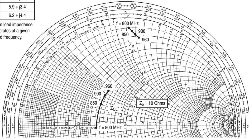
NOTE: Z<sub>in</sub> & Z<sub>OL</sub>\* are given from base-to-base and collector-to-collector respectively.
