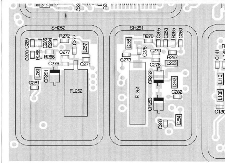
Note that even though C278 is shown as being present, in actual production radios, this component is missing. It is this position that you'll be soldering a 4.7pF SMD chip capacitor. Obtaining a 4.7pF chip cap of the right size (0402) would be useful, but if all you can obtain is the next size up (0603) then you can still make use of this, as the following photo shows:
