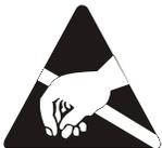
The **ESD** symbol calls attention to procedures, practices, or the like, which could expose equipment to the effects of **E**lectro-**S**tatic **D**ischarge. Proper precautions must be taken to prevent ESD when handling circuit modules.
