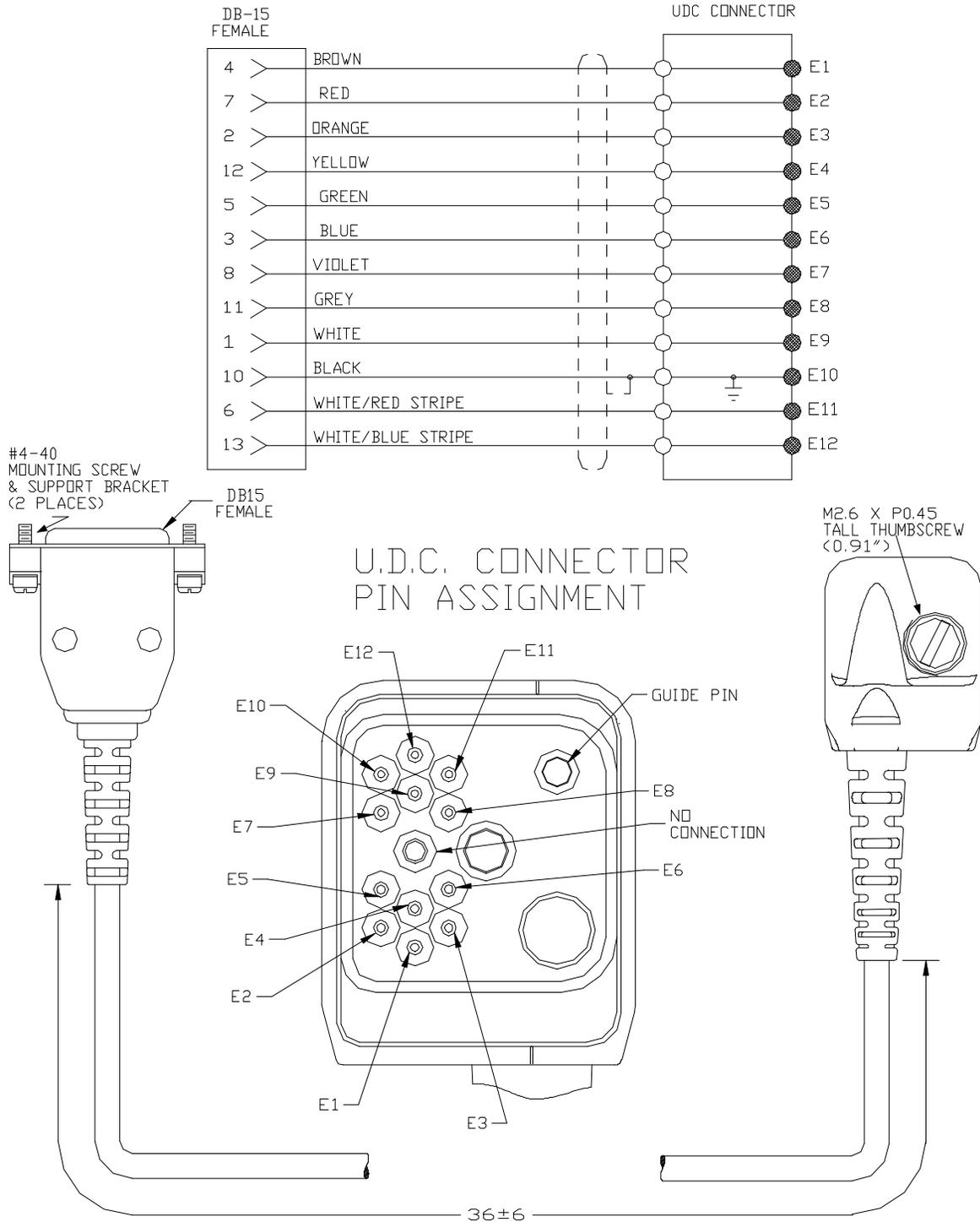
**7.7 RPM1132472/24 CABLE DIAGRAM (JAGUAR 700P, P7100, P5100 AND P7200 PERSONAL RADIOS)**
