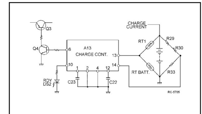
Figure 3 - Simplified Temperature Cut Off Circuit
