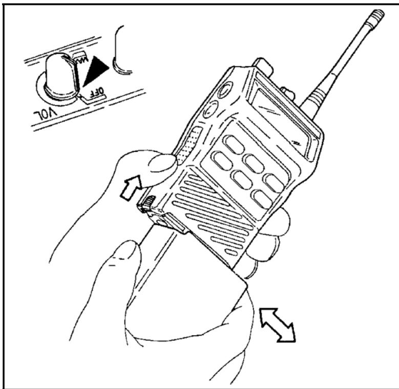
*Figure 5 - Installing And Removing The Battery Pack*
