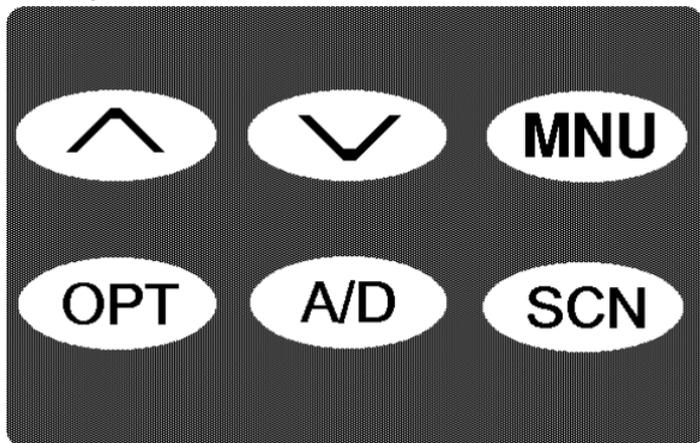
Figure 3 - M-RK II Scan Keypad
