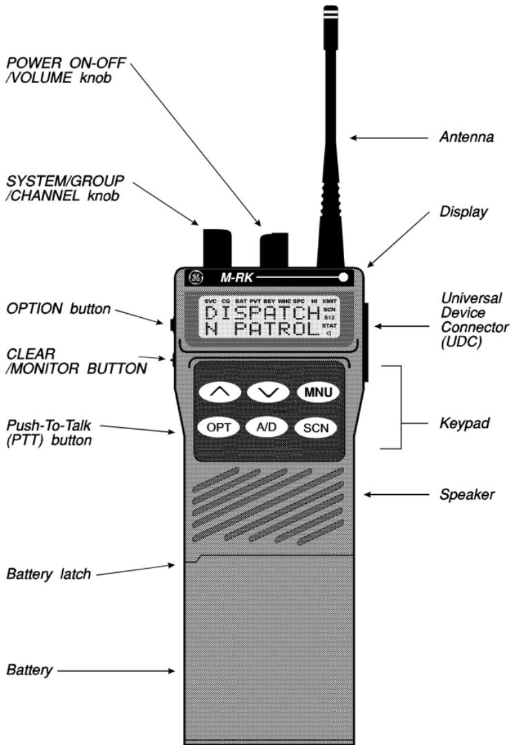
Figure 1 - M-RK II Scan Portable Radio
