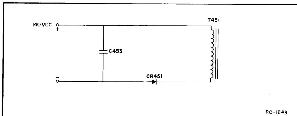
Figure 2 - Antenna Relay Supply
