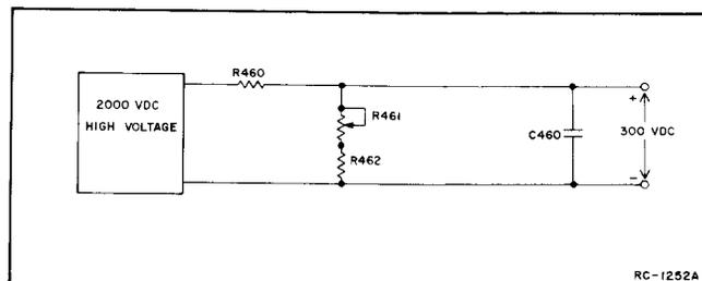
Figure 5 - Screen Voltage Supply
