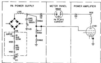
REV. E - To eliminate contact arcing between pin 8 and pin 9 on relay K454. Wires connecting to K454-7 and -8 were moved to K454-13 and -14, respectively.
