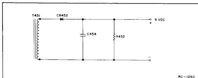
Figure 3 - Drive Relay Supply
