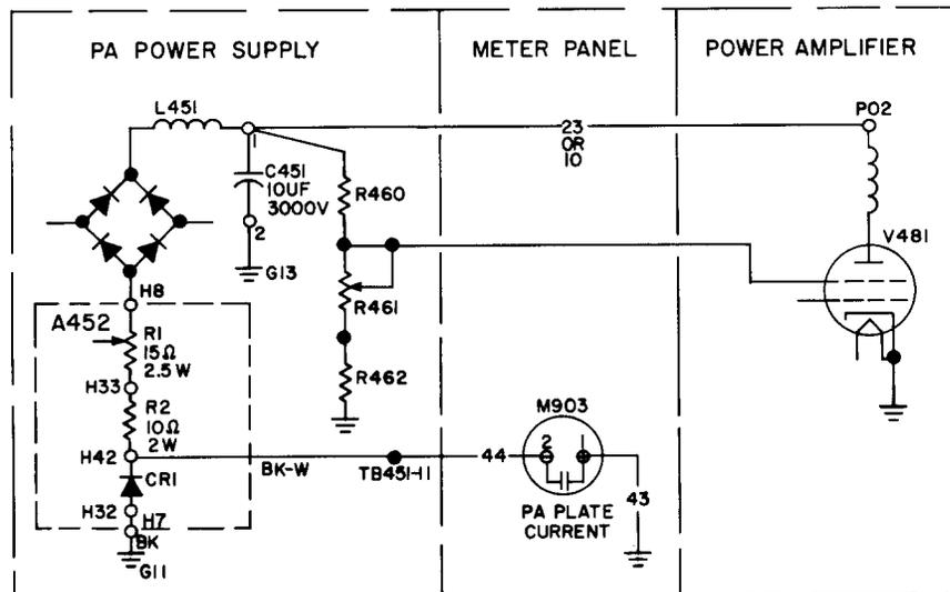
Figure 7 - PA Plate Current Metering Circuit
