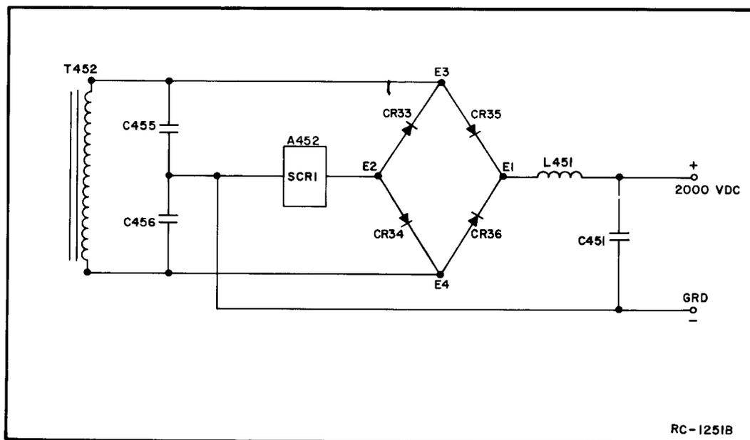
Figure 4 - High Voltage Supply
