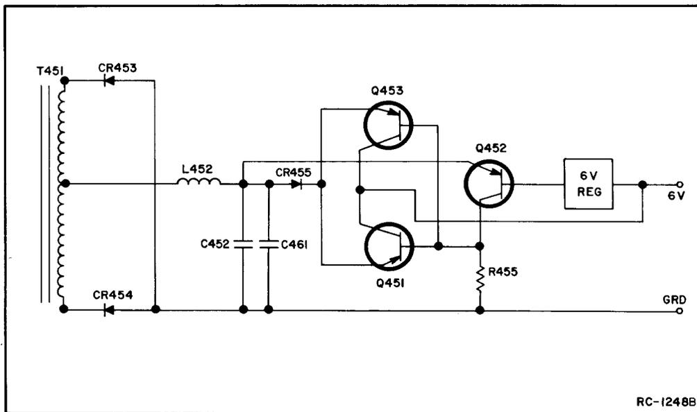
Figure 1 - Filament Supply
