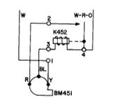
REV. D - To eliminate PA plate meter damage if 2000 VDC line becomes shorted. Added CR1 to A452 and changed meter connection point.
