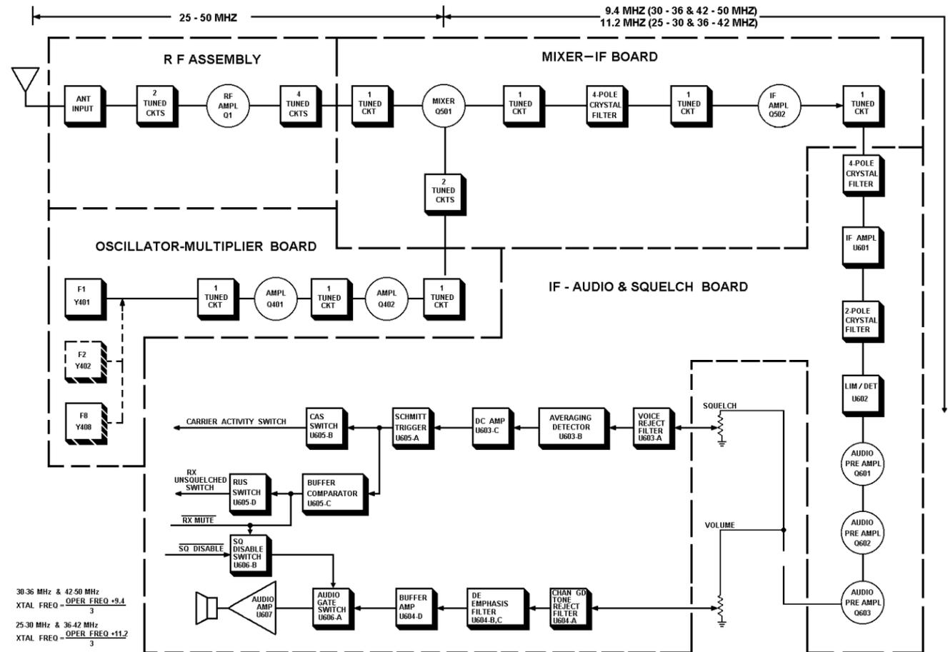
Figure 2 - Receiver Block Diagram
