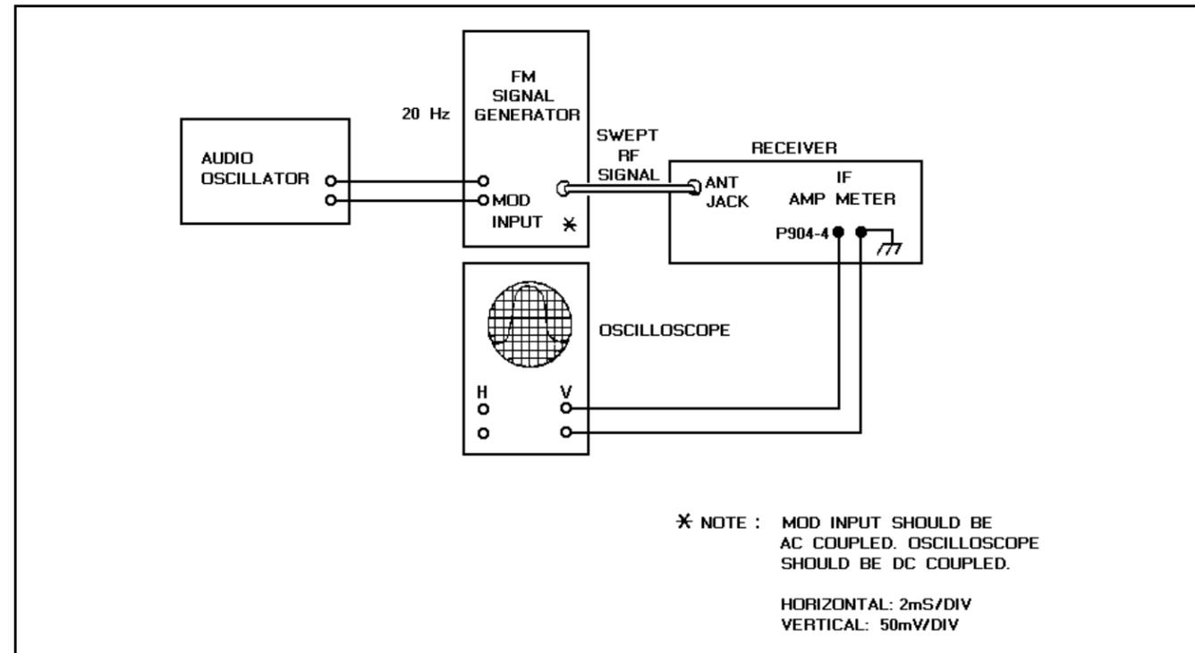
Figure 6 - Test Setup for 20 Hz Double-Trace Sweep Alignment
