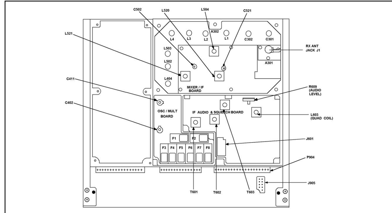
Figure 5 - Test Points And Alignment Controls
