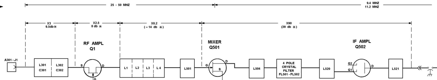
NOTE: REMOVE ICOM TO MEASURE VOLTAGE ON GATE OF MIXER.
