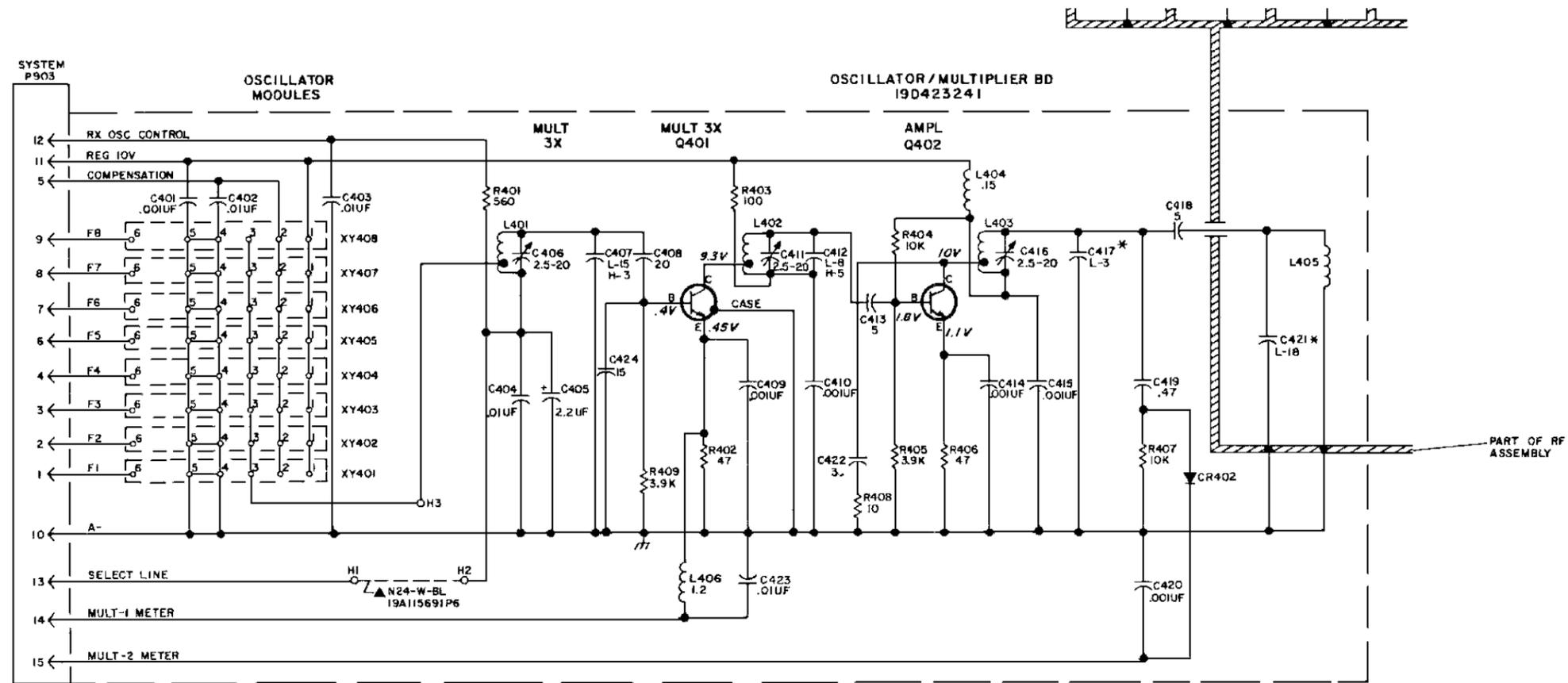
▲ THESE COMPONENTS ARE USED TO ADAPT A STANDARD MASTR II RECEIVER TO OPERATION AS AND WITH A DUAL FRONT END. THESE COMPONENTS SHOULD BE IGNORED IN THE STANDARD RECEIVER. BOARDS IDENTIFIED BY A RED DOT HAVE BEEN MODIFIED FOR DFE OPERATION PER MOD KIT 19A129750G1 OR G2.
