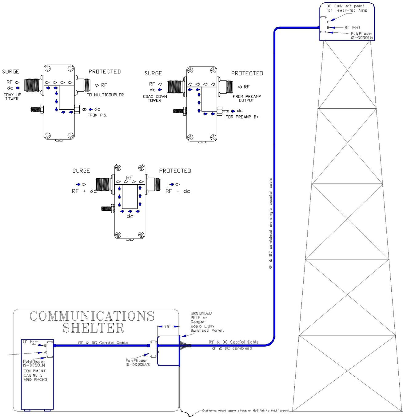
**Figure 10 - Tower -Top Amplifier & DC Power Insert/Pick-Off Connections**
