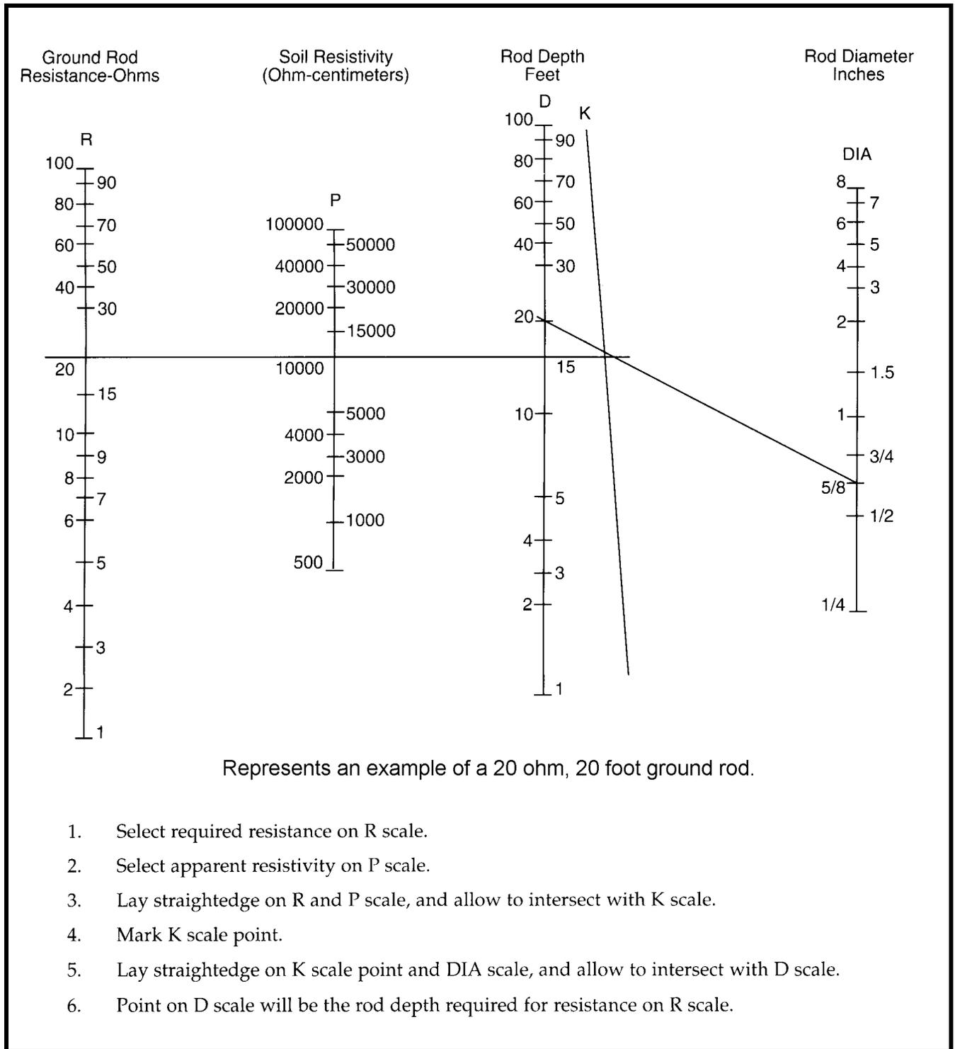
**Figure 4 -Grounding Nomograph**
