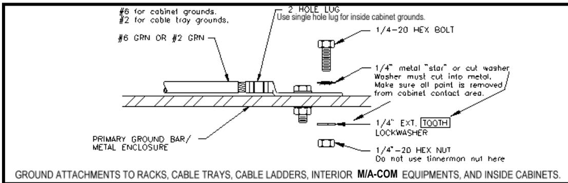
**Figure 21 - Ground Attachment Methodology**
