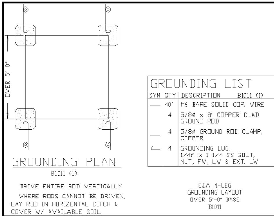
Figure A-3 Four Leg Tower Grounding Kit
