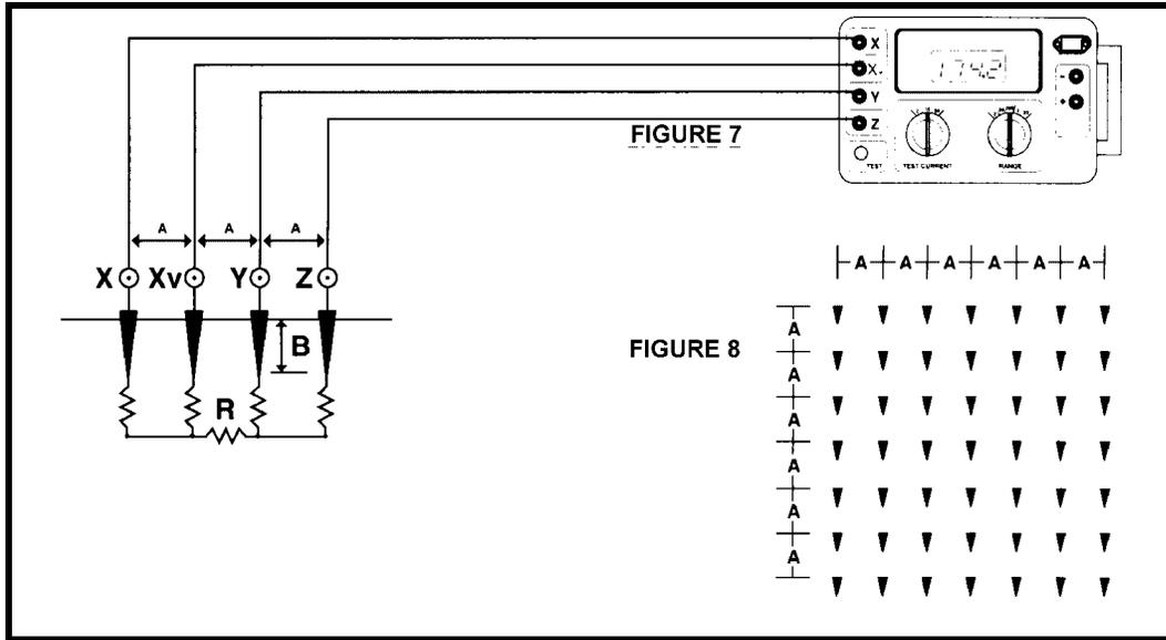
**Figure 3 - Soil Resistivity Measurements Using the Model 4500**
