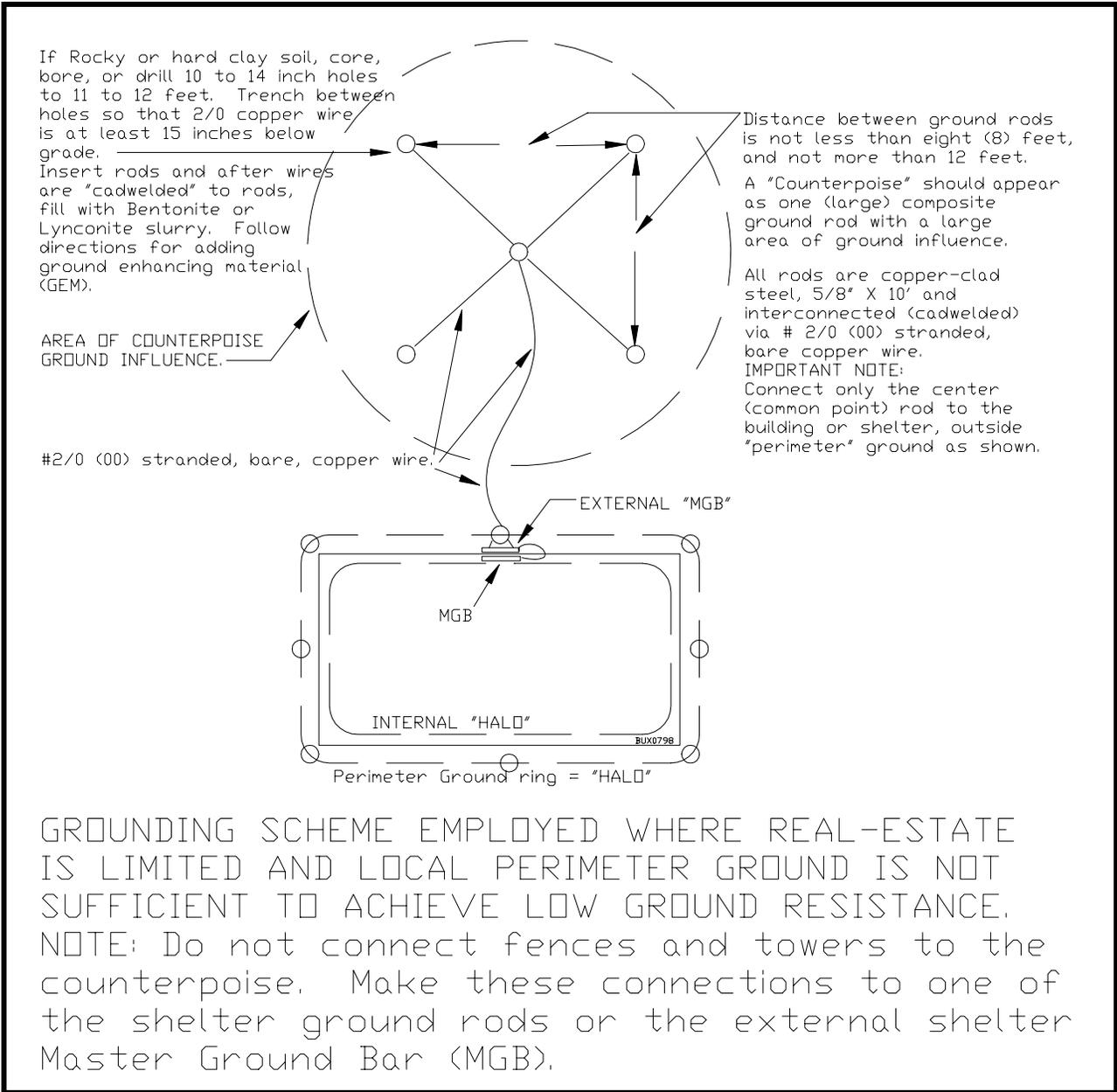
**Figure 13 Counterpoise Ground Diagram**
