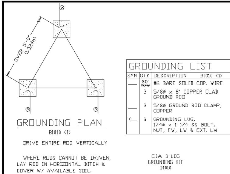
**Figure A-1 3 Leg Tower Grounding Kit**
