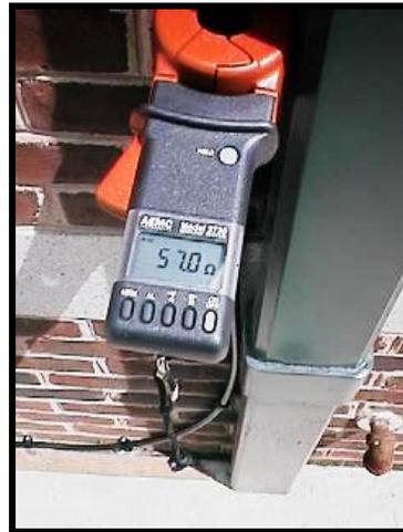
Figure 5 - Ground Measurement Using the AEMC Model 3730
