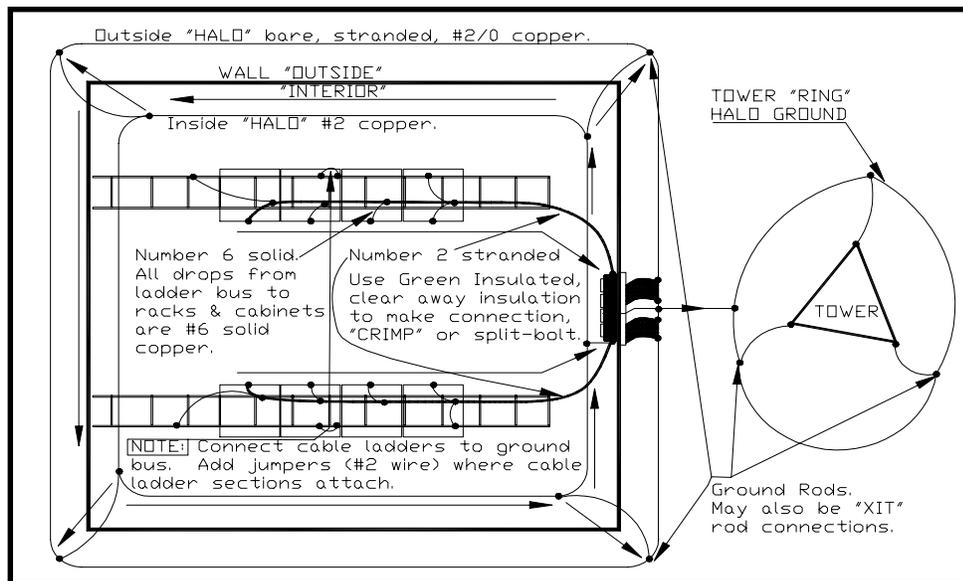
Figure 9 - In-Building Halo Ground Ring
