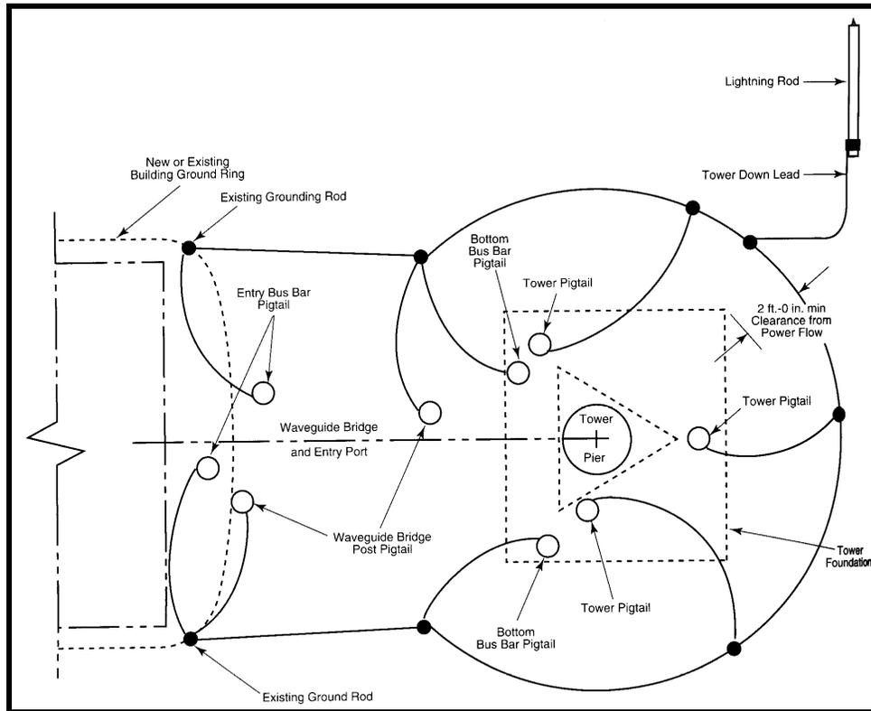
Figure 8 - Tower Halo Ground Ring
