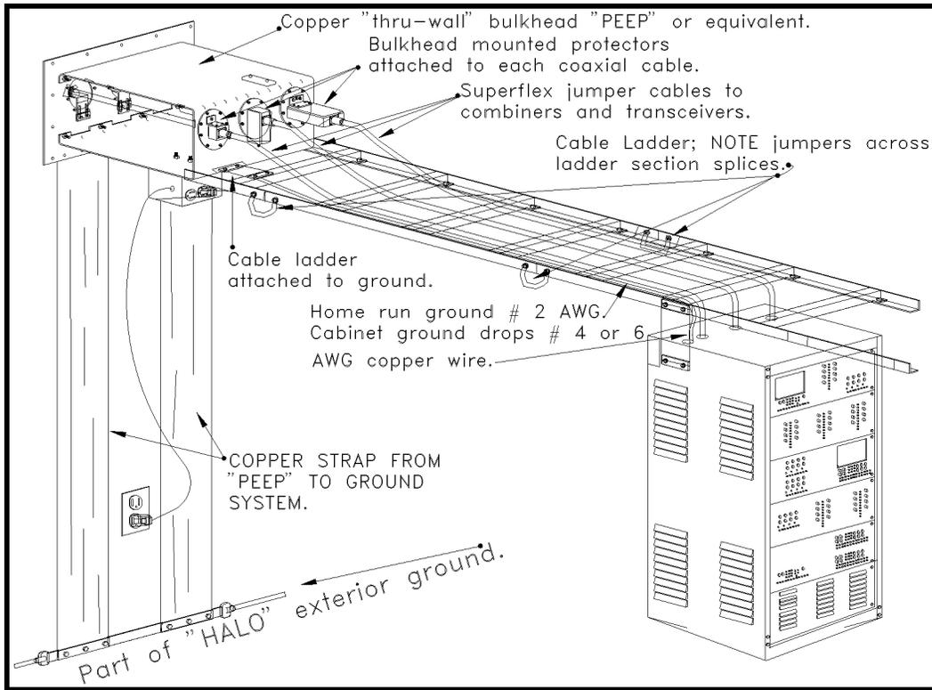
**Figure 20 - Ground Attachments in Installation**
