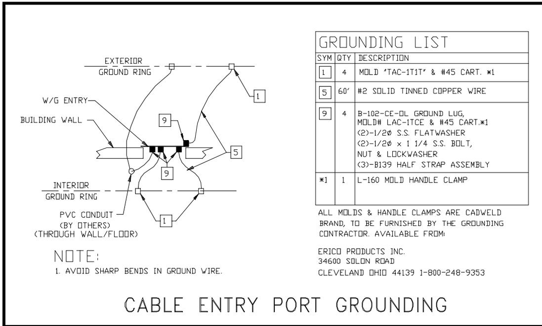
Figure A-5 Cable Entry Port Grounding Kit
