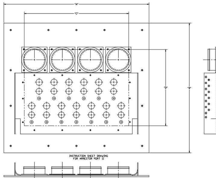
**Figure 18 - The ANDREW Integrated Cable Entry/Grounding System**
