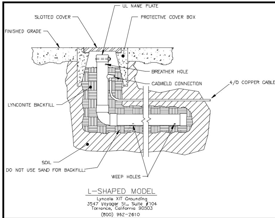
**Figure 24 - Installation Instructions for XIT Lyncole L-Shaped (Calsolyte™) Ground System**
