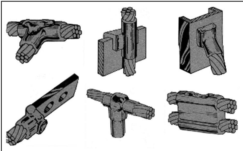
Figure 14 - Typical "Exothermic" Welds Made Using the Cadweld Method.
