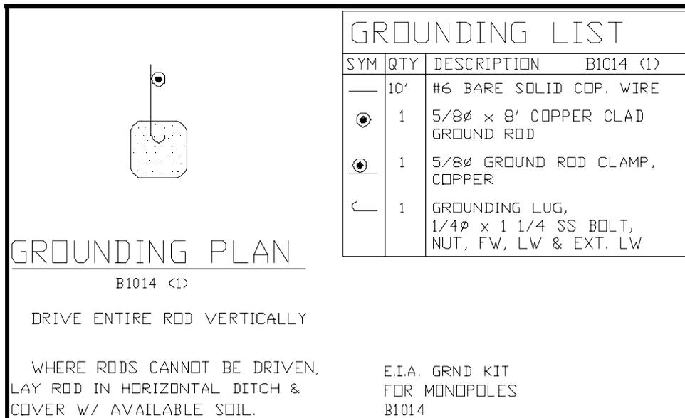
Figure A-4 Monopole Tower Grounding Kit
