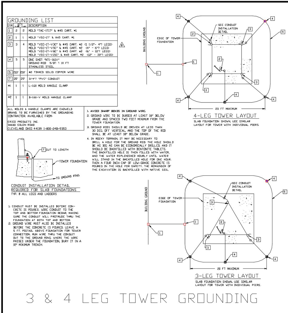
Figure A-9 3 and 4 Leg Tower Grounding Kit
