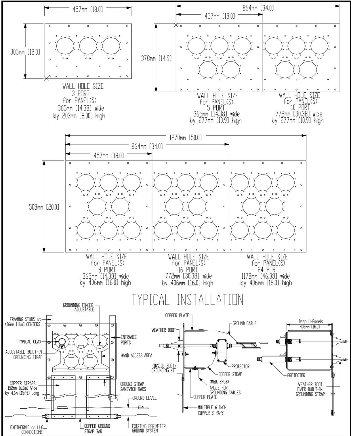
**Figure 17 - Typical Installation Cable Entry Panel(s).**
