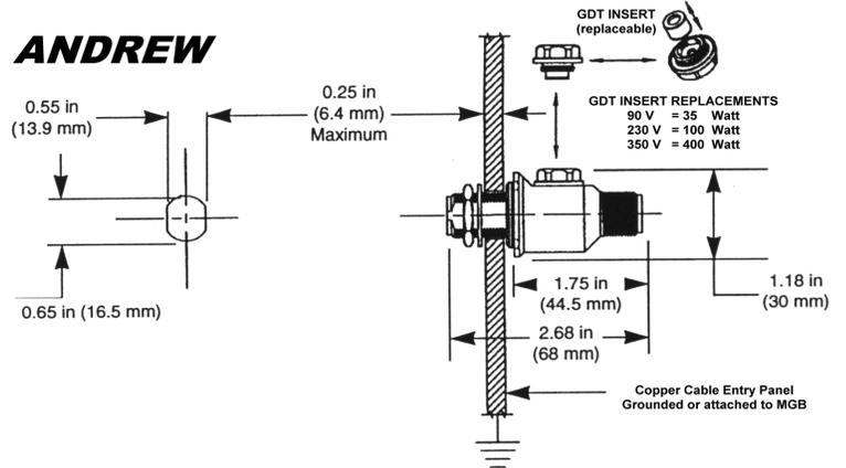
The Andrew Gas Discharge Tubes Surge Arrestors shown here have replaceable GDT inserts. This has the advantage of being able to replace the GDT insert without removing the arrestor from the coax cable or the ground bus panel.
