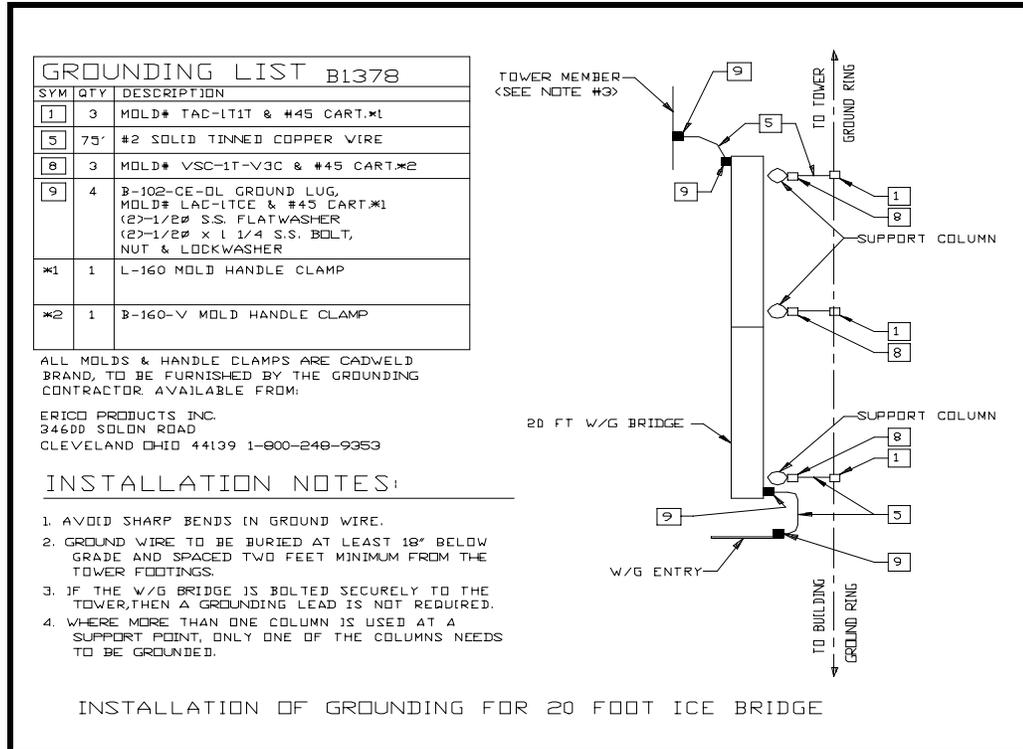
Figure A-7 20' Ice Bridge Grounding Kit
