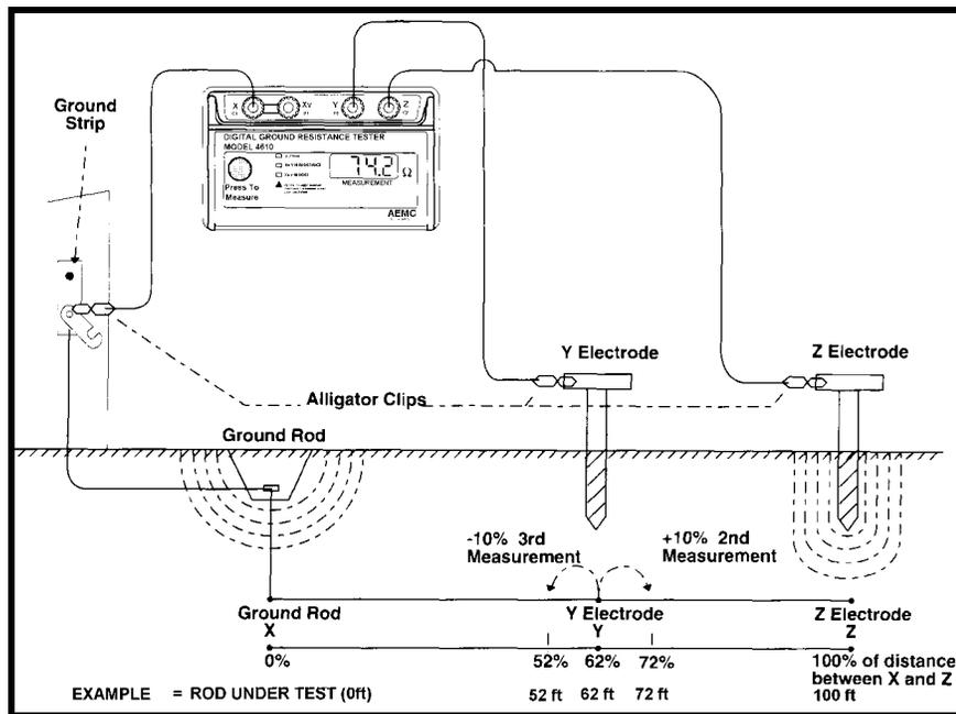
Figure 6 - “62 Percent Method” Ground Measurements
