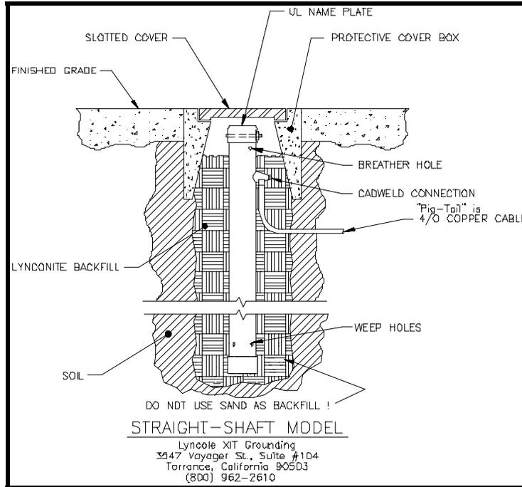
**Figure 25 - Installation Instructions for Straight Shaft (Calsolyte™) Ground System**
