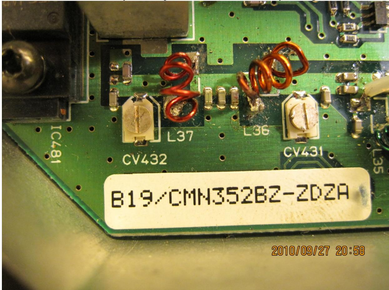
Figure 5. Receiver pre-selector inductors L436 and L437, home made and initially preset at 3 wire diameter spacing.
