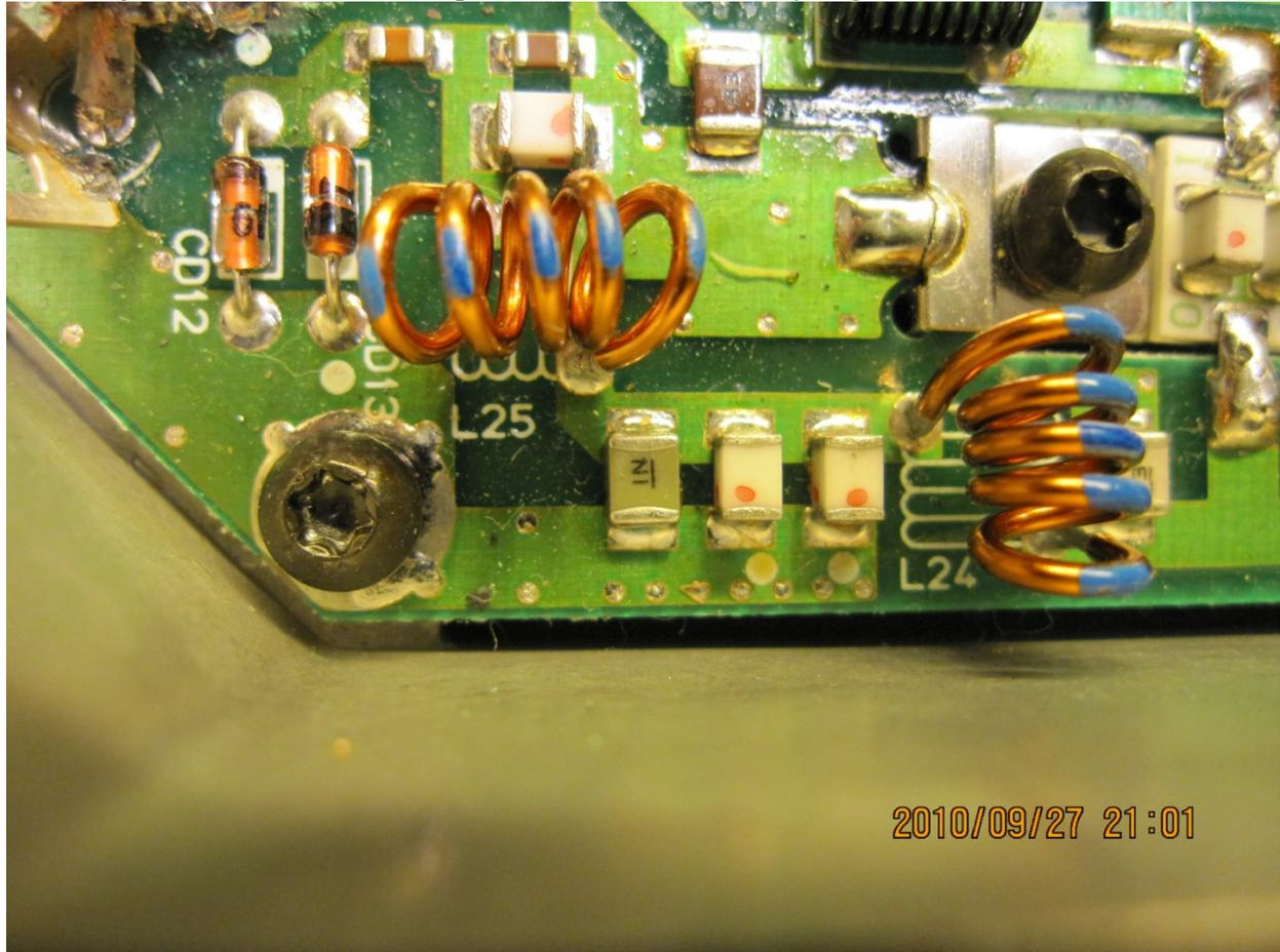
Figure 7. Receiver  $\frac{1}{4}$  wave line. Presetting of L24 end turns at 1 wire spacing and the middle turns at  $\frac{1}{2}$  wire spacing. Set L25's end turns at 2 wire spacing and the middle turns at 1 wire spacing.
