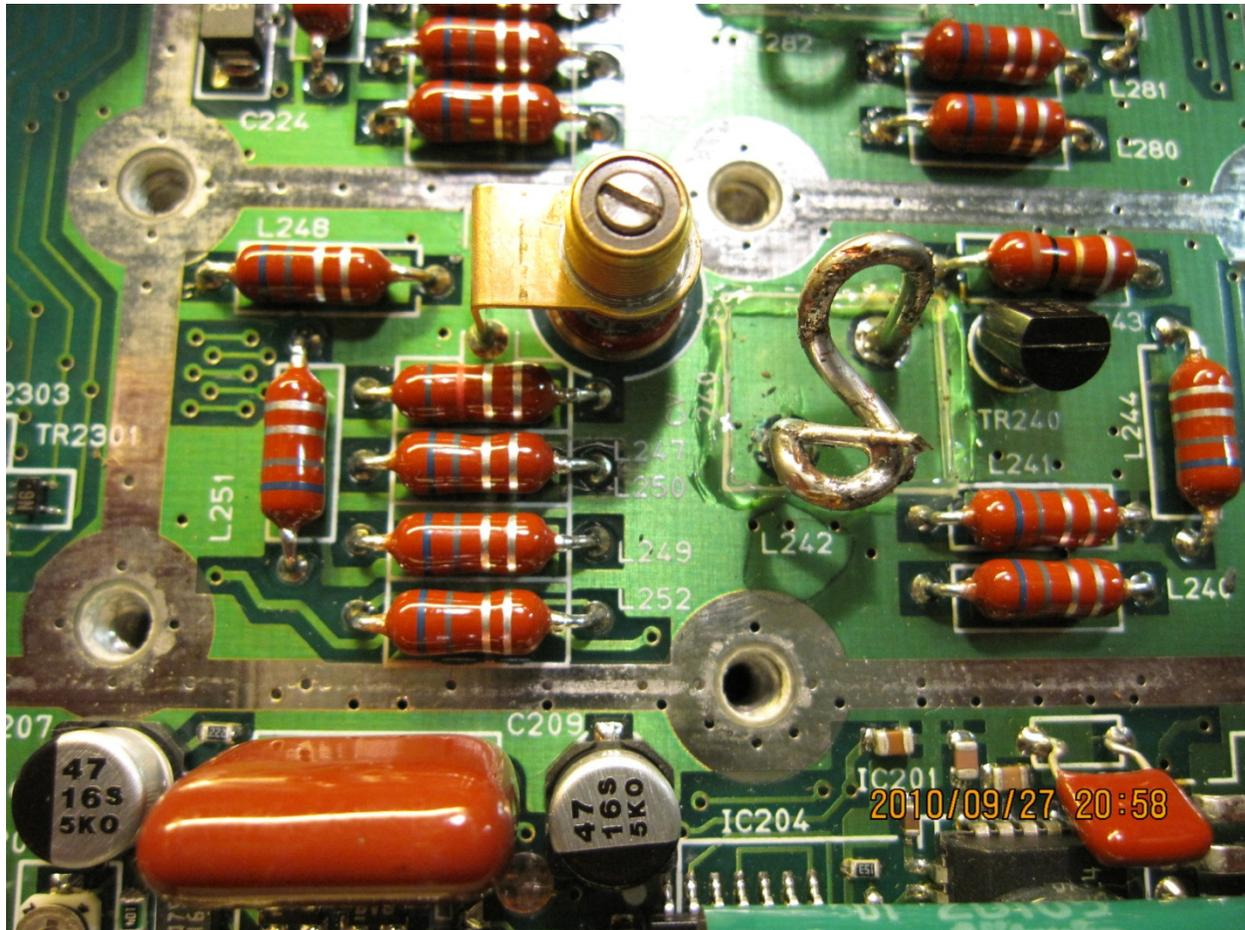
FIGURE 1. receive, spread VCO inductor L242 while adjusting RX VCO tuning capacitor, CV240 for receive VCO lock.
