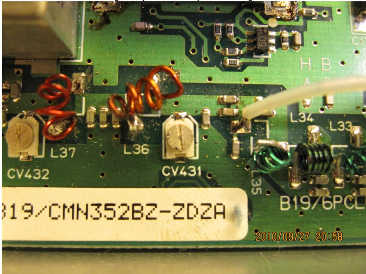
FIGURE 3B. L35 lifted on tracking filter output end.
