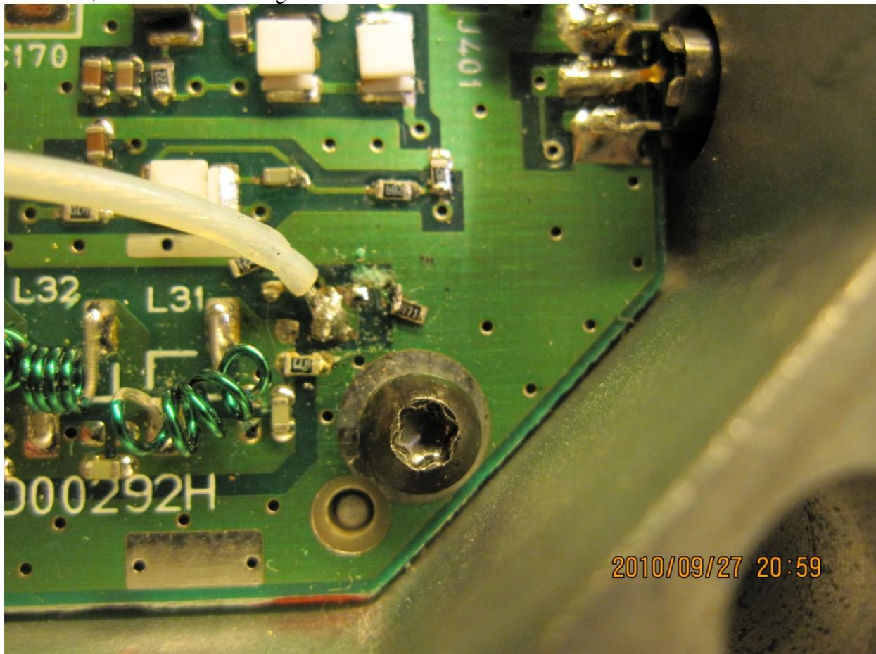
FIGURE 3A, Tracking band pass filter input side is isolated by lifting R411 to R413 to remove the tracking filter from the circuit.
