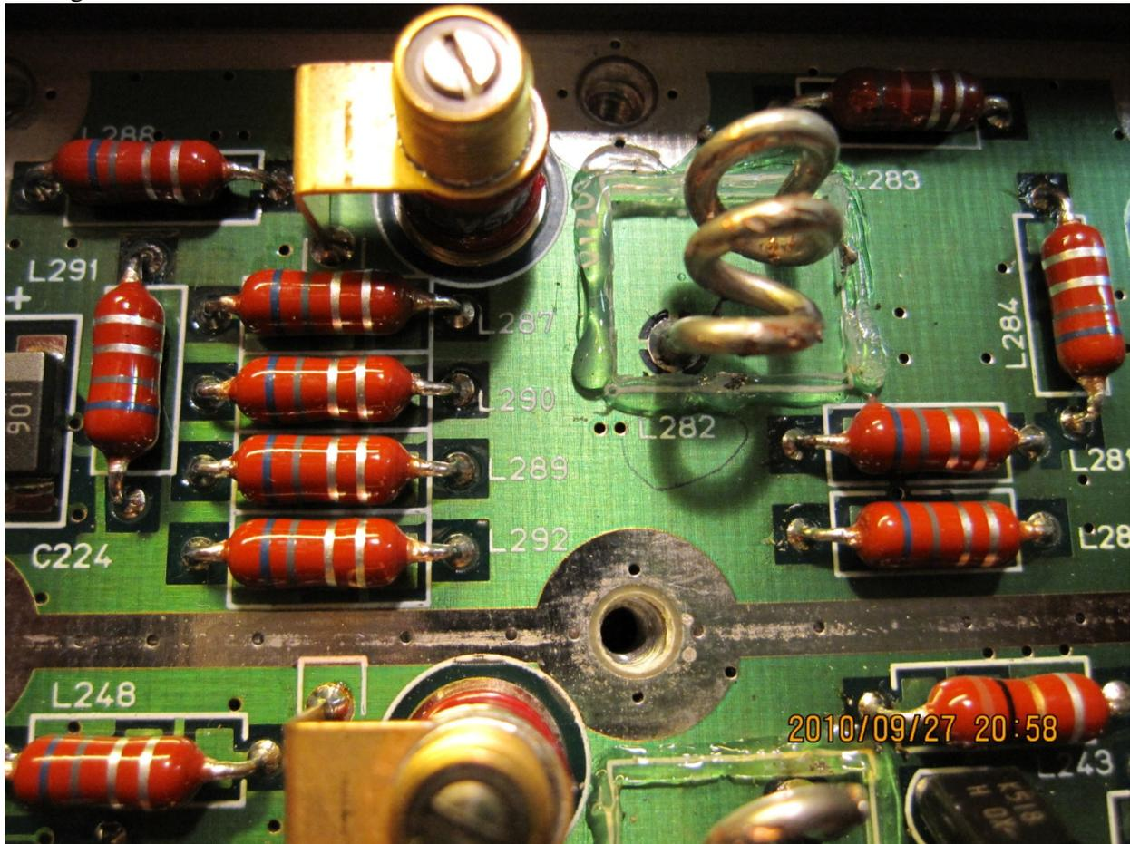
FIGURE 2. L282 Spread TX VCO coil and adjust TX tuning capacitor CV280 for transmit VCO lock.
