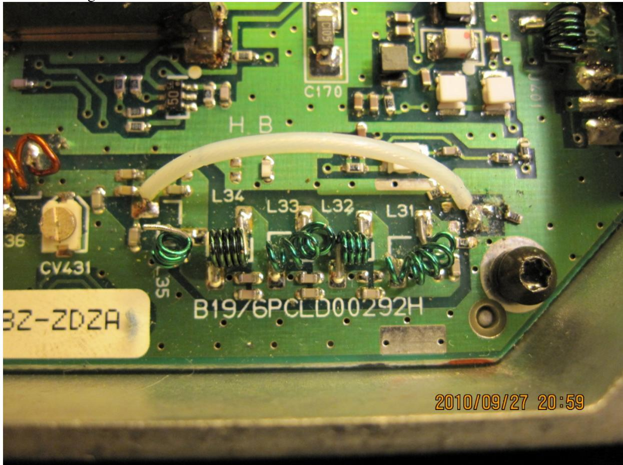
Figure 4, tracking rx band pass filter, L31 through L34 bypassed.
