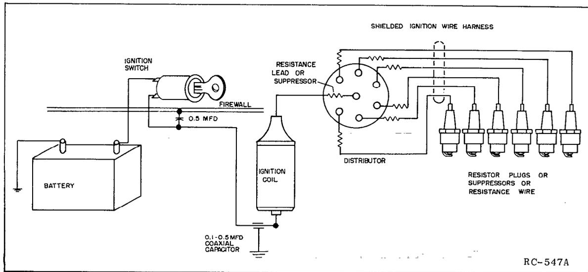
Figure 2 - Ignition Circuit with Noise Suppression Components
