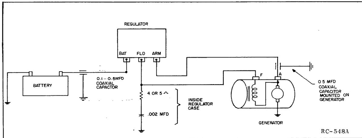
Figure 3 - Generator Circuit with Noise Suppression Components
